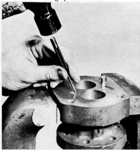
Peening over check valve seat
