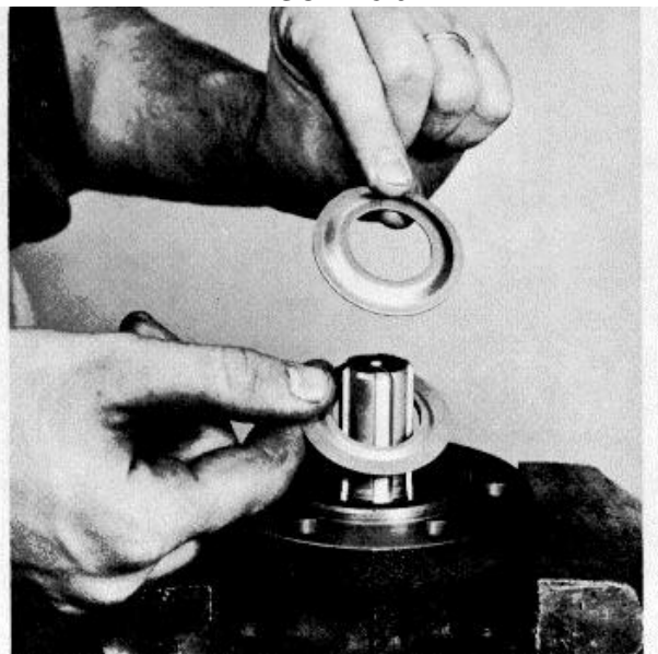
Installing bearing seal and shield FIGURE 6-9
