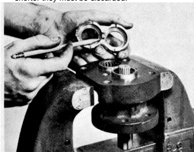
Inserting socket seals FIGURE 6-11
